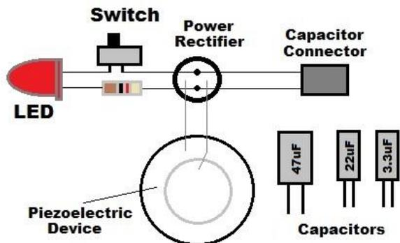
will connect or disconnect our LED from the circuit. The power rectifier converts the alternating wave produced by the piezo to a direct current for use in our system. The capacitors will be used to store energy and the capacitor connector is where we can connect our capacitors to the circuit.
