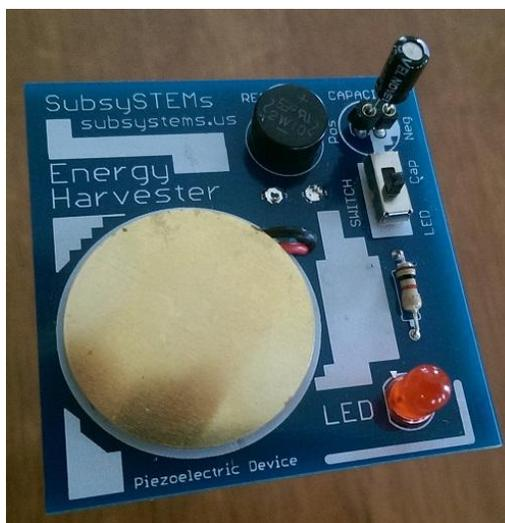
The piezo is generating energy that the LED is using to light. Let's use our system to store this energy.
