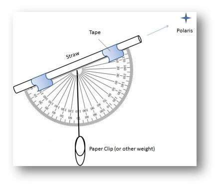
On a clear night, go outside and sight in Polaris through the straw. Read the angle that the string marks on the protractor. Use the scale that is 0 to 90 degrees. Now, subtract the angle from 90 degrees to get the elevation of Polaris. This is your latitude. In the picture, the string is showing an angle of 70 degrees. When we subtract this from 90 degrees, we arrive at latitude 20 degrees.
