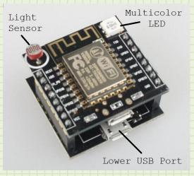
IoT. He includes a lower USB port for power and programming (the upper port can be used for power only). There is a light sensor for input and a multicolor (Red/Green/Blue) LED (light emitting diode) for output. There are also 3 pushbutton switches. On the bottom board there are two labeled RST and FLASH and are used for programming. The switch on the top board is for user input.
