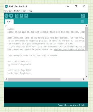
When you open the sketch, the code will appear in the code window. The Blink example will just load the code to blink the LED on the Arduino board. Let's hook up the board and get it ready to receive code. First, let's make sure that the IDE is set to the correct board. The board included in your kit is an Arduino UNO. From the menu, select:
