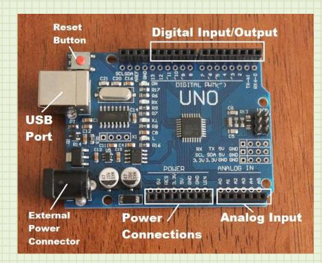
The UNO can be powered from the USB cable or from an external supply. We will be using the USB connection for both power and for uploading programs to the board.
